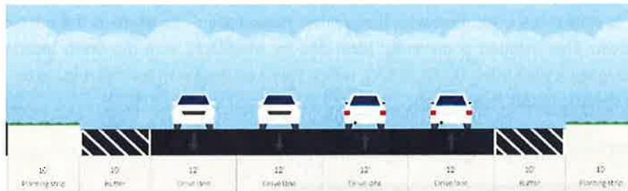
FIGURE 1: ROUTE 1 EXISTING TYPICAL SECTION
