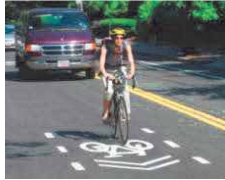
Sharrows Indicating Bicyclists can Ride in Center of Lane Location: Brookline, MA Source: MAPC
