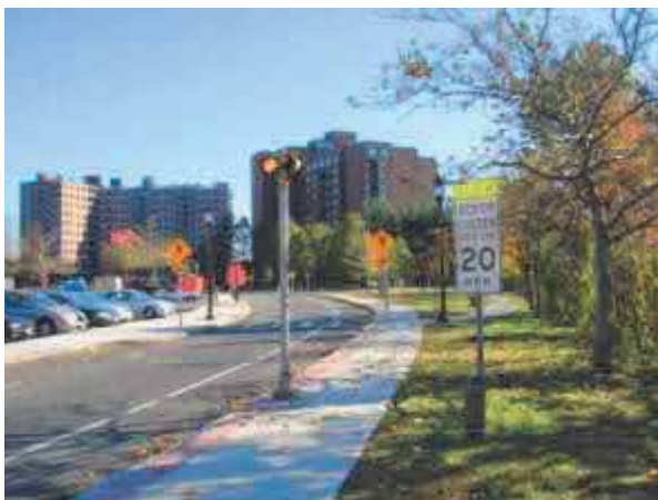
Pedestrian Activated Flashing Crosswalk and Signage Location: Medford Square, MA Source: Paul Reavis, Wakefield Town Planner
