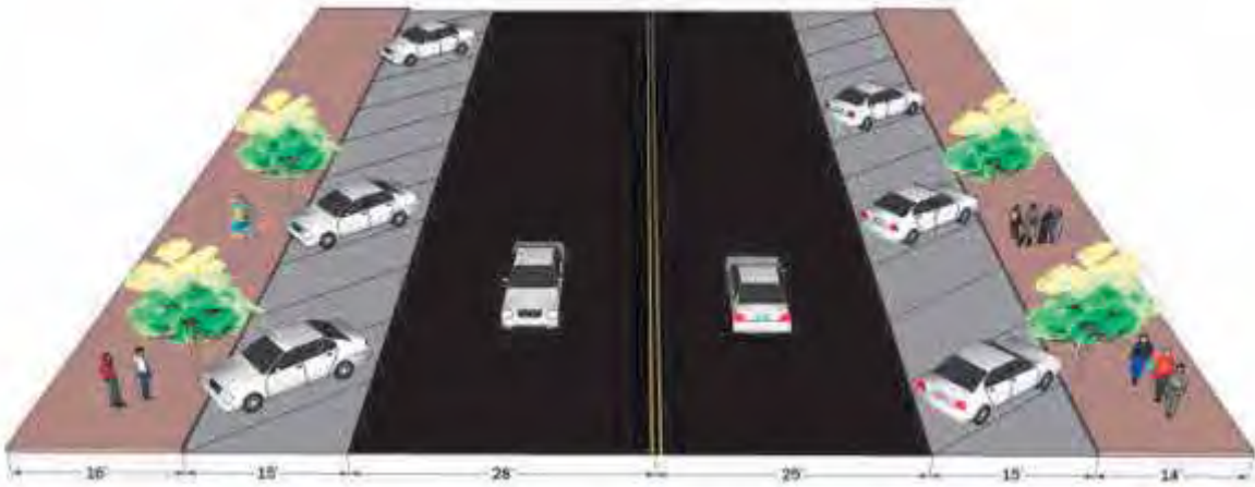
Existing Condition: Angle Parking, Wide Vehicle Travel Lane, No Bicycle Lanes
