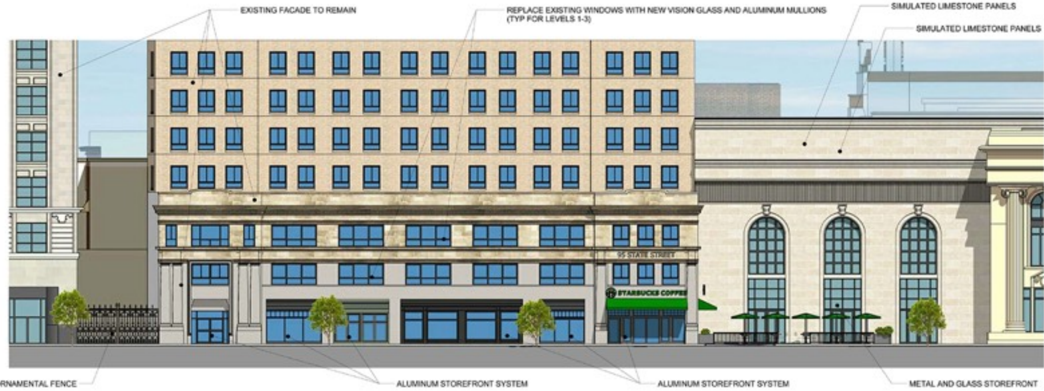
ENLARGED STATE STREET ELEVATION (PART 1 OF 2)
