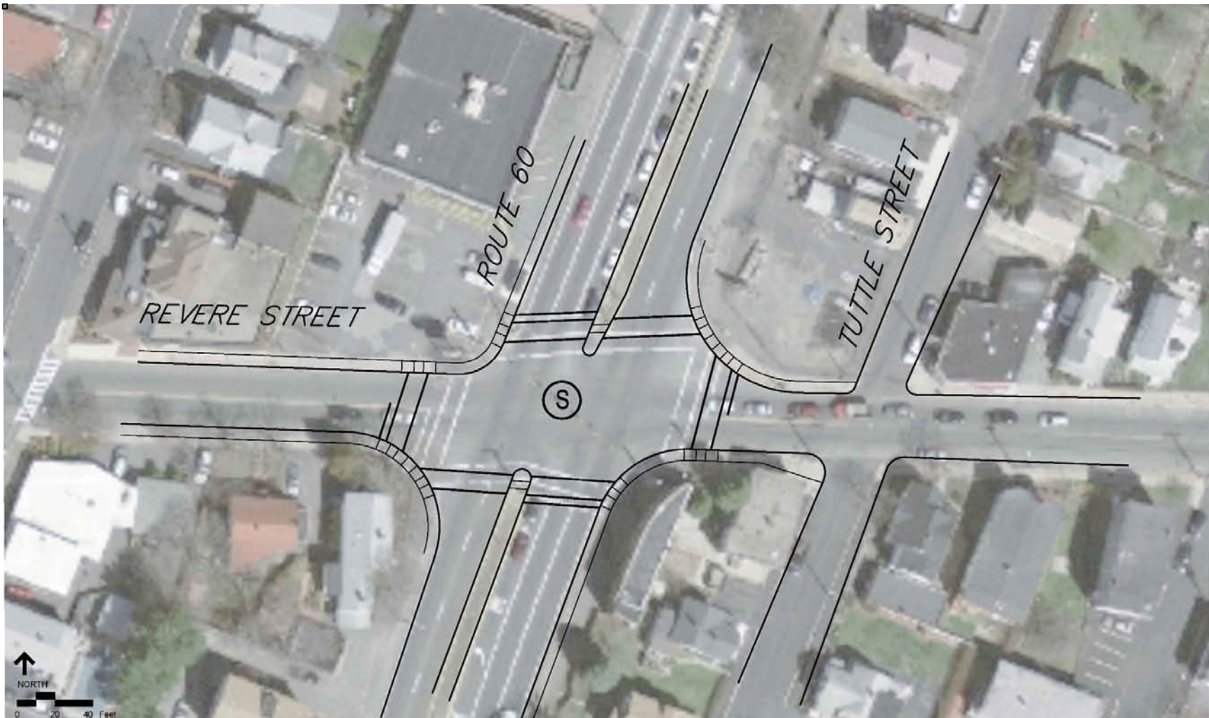
Figure 26 – Proposed Improvements at Route 60/Revere Street
