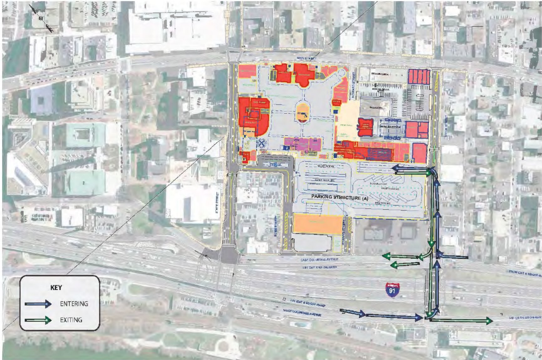
Figure 10 – Traffic Flow – Bus and Delivery Truck Access
