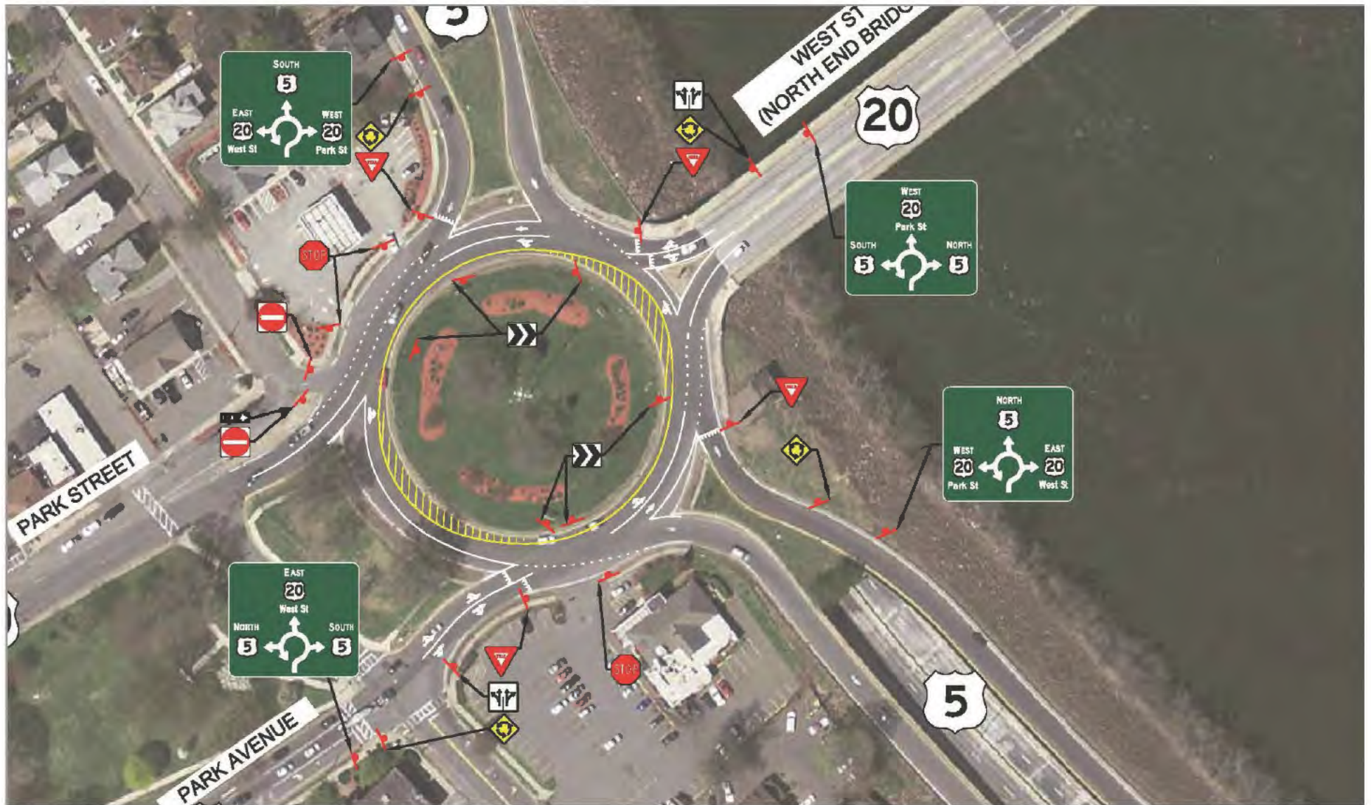
Figure 8 – Mitigation Measure Examples – North End Rotary – Proposed Pavement markings and Signage
